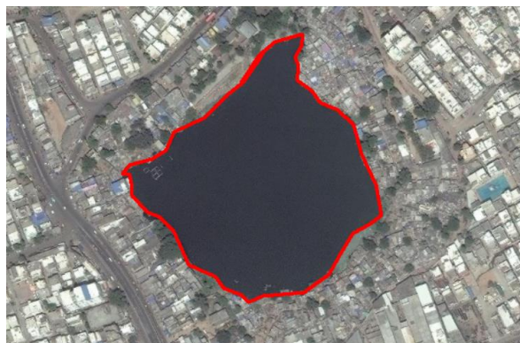
Figure 2.12: Digitization of polygon of a pond
