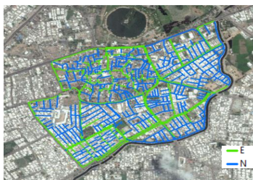
Figure 3.3: Existing and new proposed pipelines
